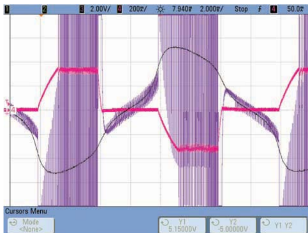
Figure 10 The loading for a loaded motor is more in line with the current it is receiving.
