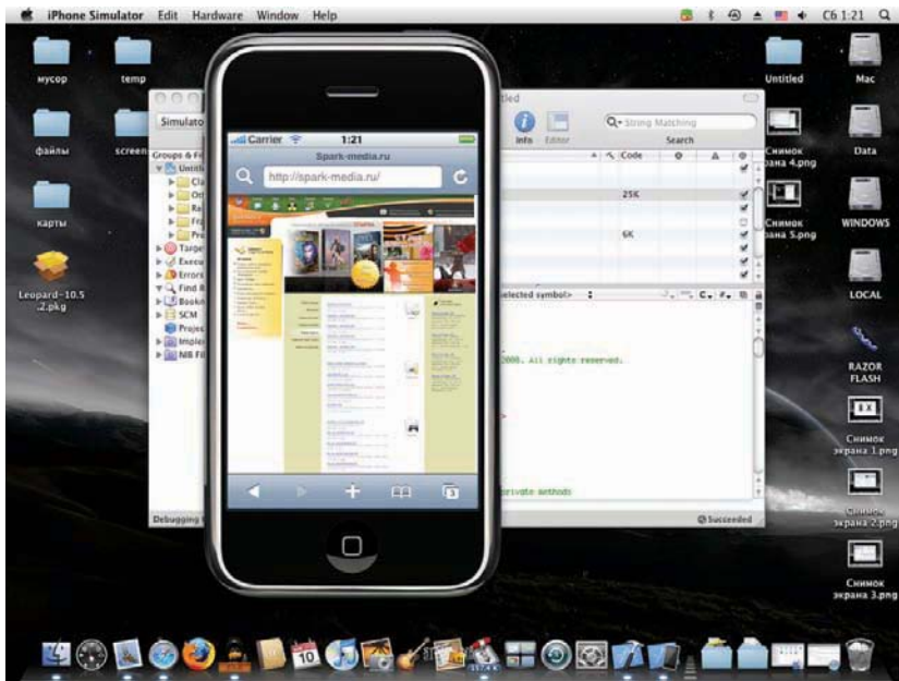
Figure 3 An SDK for an iPhone allows an application developer to write and debug software without executing it on the device.
